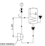
Figure 4.6: Pressurisation tank installation sketch
