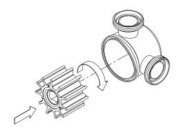
Before the impeller (02) is mounted, it should be lubricated with grease. For food-processing applications, use health-safe grease.
