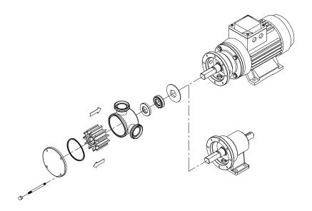
CAUTION! When mounting the new seal, plunge the parts and seals in soapy water to facilitate sliding of both the stationary and the rotary parts.
