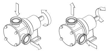
Start the pump motor briefly. Ensure the pumping direction is the right one. If the pump operates in the wrong direction it may cause severe damage.
