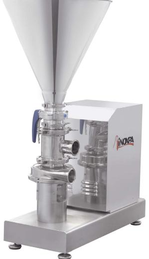
It is important to keep low pressure at the suction and at the dishcrage sides of the blender. Avoid cavitation. Thus a feeding pump must be provided only for the applications that really require it (considerable pressure drops at the suction side, high viscosity products, etc.), please, keep in mind that the suction capacity will decrease.
